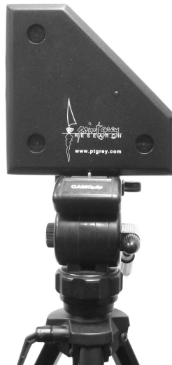
Figure 6.1: The Digiclops camera used for triocular video acquisition.
